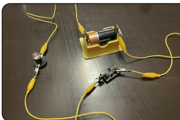
You can even build a switch into your circuit so you can open and close the connection that allows electrons to flow and power the bulb.
