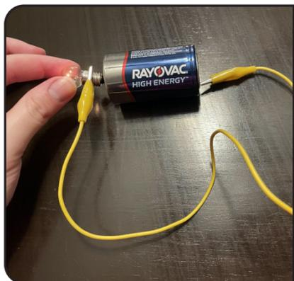
The most basic circuit includes a power source and something to connect it back to itself, like a battery powering a lightbulb. The battery can only power the bulb if there's a full loop for the electrons to flow from an area of negative charge to an area of positive charge (more electrons to a place with fewer electrons).
