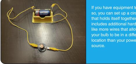
If you have equipment to do so, you can set up a circuit that holds itself together and includes additional hardware like more wires that allow your bulb to be in a different location than your power
