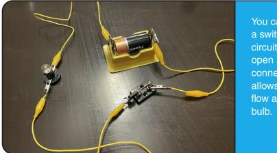
You can even build a switch into your circuit so you can open and close the connection that allows electrons to flow and power the
